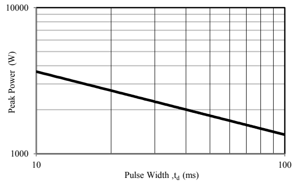
Fig. 4 - Peak Pulse Power Rating Curve
